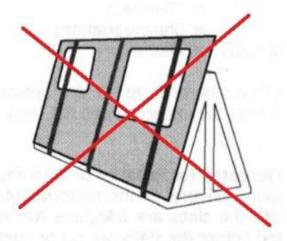
Never lay an ASCALE slab or piece onto a shorter piece of stone or product. The ASCALE should always be flush and fully supported prior to strapping and securing for transport.
