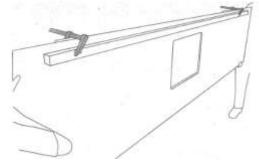
3. When laying your ASCALE slab onto a table ensure the entire cut piece is spine supported by the edge of the table prior to rolling the piece onto it. Ensuring both ends are equally moving into place.
